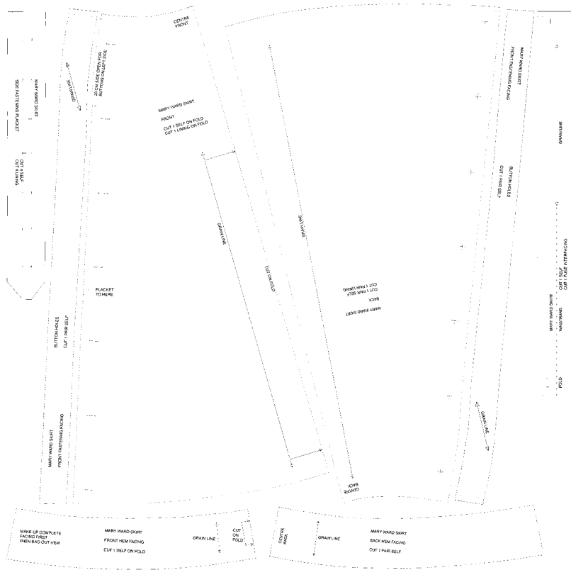
Figure 10.6 The pattern inspired by Mary’s convertible cycling skirt consists of eight pieces: front, back, front side facing, back side facing, hem front and back, side strap and waistband
