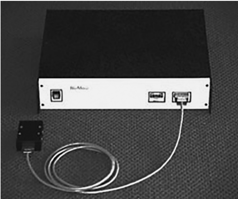
Figures 7.1–7.3 The BioMuse, system cable and 8-way breakout box; the underside of the BioControl WPM unit; Infusion Systems BioFlex EMG sensor.
