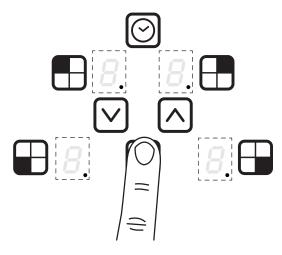
**5** Press the on/off key to switch the appliance on
