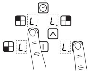
Press the on/off key to switch the appliance on. Child lock is now deactivated.
