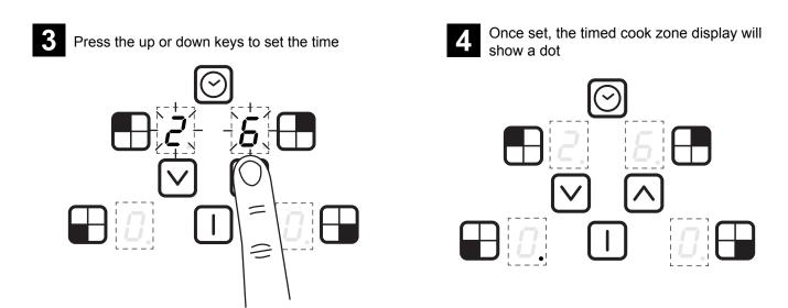
The timer indicator in the display stops flashing and is not displayed. Operation of a timer is shown by a stationary dot in the cook zone display for the timed cook zone.
