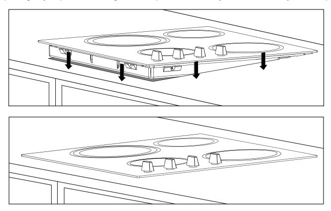
**Note**; The worktop cut out dimensions are critical and will affect the performance of how the push fit system works. The nominal dimensions are shown on the hob cut out table and must be fabricated to a tolerance of +2.0mm -0.0mm. The effectiveness of the system will vary depending on the accuracy of the worktop cut-out dimensions.
