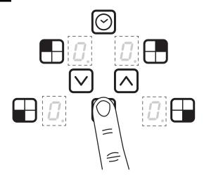
Remove fingers and touch the down key. The child lock should switch off
