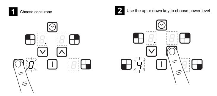
When the cook zone selection is finished after 10 seconds, a beep sounds and all the heater displays that were dimmed show the power levels with normal brightness.
