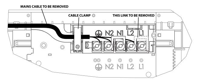
Fit 3 phase mains cable in terminal block as shown in table below;
