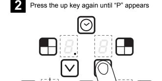
For quick operation, with the cook zone power level "0", press the down key then the power level will raise straight to "9". Press the up key and display will show the Power Boost level.
