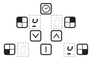
The above "U" symbol appears when a zone has been activated but no pan has been placed on the cook zone. If the "U" symbol does not disappear when a pan is placed on the zone it indicates that the pan is not suitable for induction cooking.
